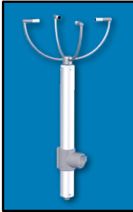
2D – 15cm Sonic Anemometer
