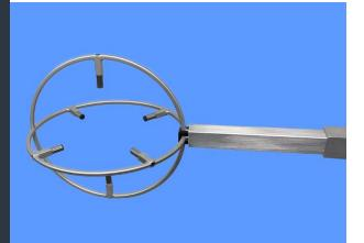
The 'Vxsp' style Ultrasonic Anemometer is a 3 axis, 3d, 15 cm, scientific Ultrasonic Anemometer This design incorporates a full circle on both axes which strengthens the arms for more durability. Like the "Vx" probe, it is designed for flux measurements in plant and forest canopies where wind speeds are extremely low, and directions are highly unpredictable.
