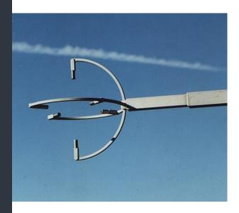
Compact design for turbulent flux measurements in plant and forest canopies where wind speeds are very low and directions highly unpredictable.
