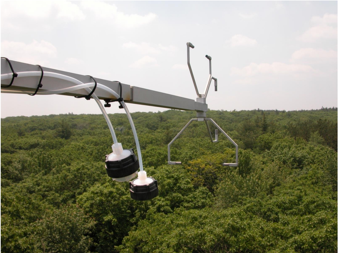
Figure 2: ATI K-Style sonic anemometer mounted to the end of the arm on the EMS tower.
