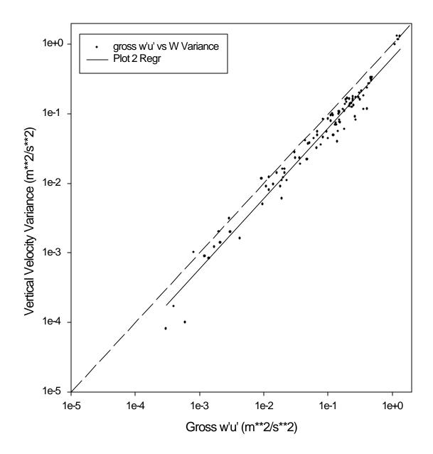
Figure 4. Plot of vertical velocity variance versus gross momentum flux ( $r^2 = 0.97$ ). The dashed line is a 1:1 fit; the solid line is the line of regression.
