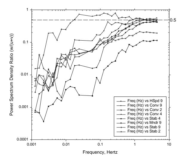
Figure 1. Power density ratio [P(w)/P(u+v)] for eight sets of spectra selected to represent a wide range of stabilities and wind speeds.
