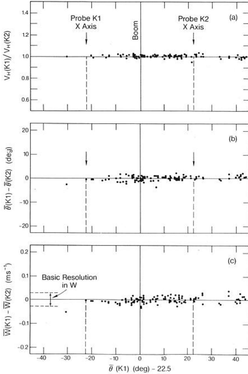
Fig. 5. One-minute horizontal wind vectors, vector directions and vertical winds measured by probes K1 and K2 in the configuration shown in Fig. 2.
