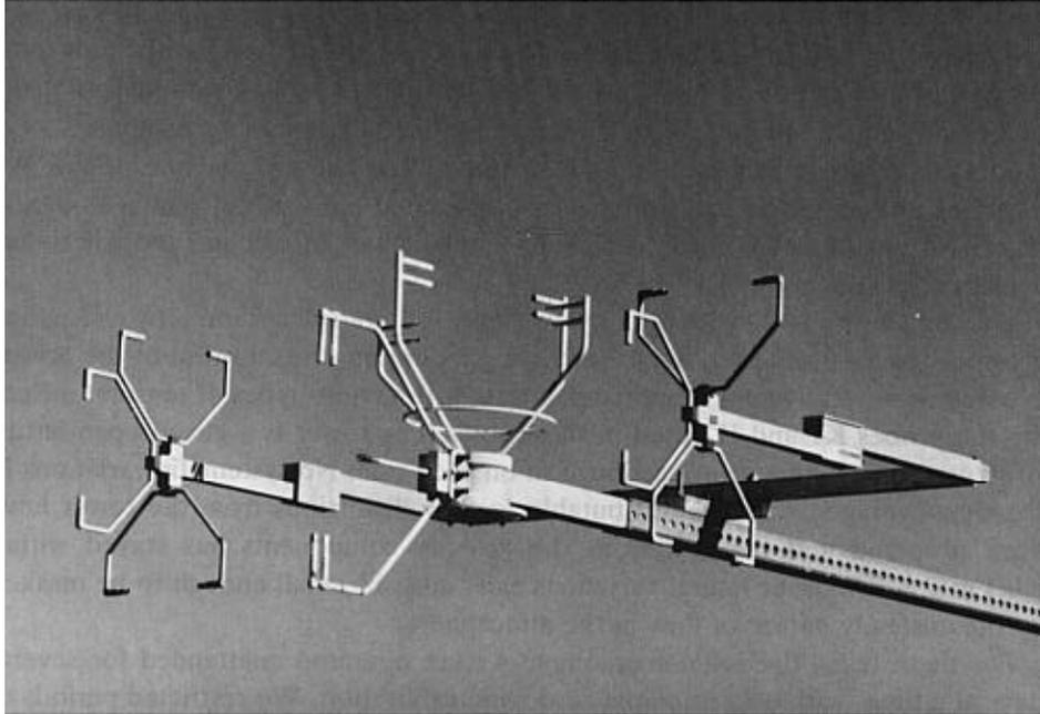
Fig. 1. Line-up of sonic anemometers used in the tests. Left to right: New K1 probe, BAO probe, and new K2 probe (inverted).
