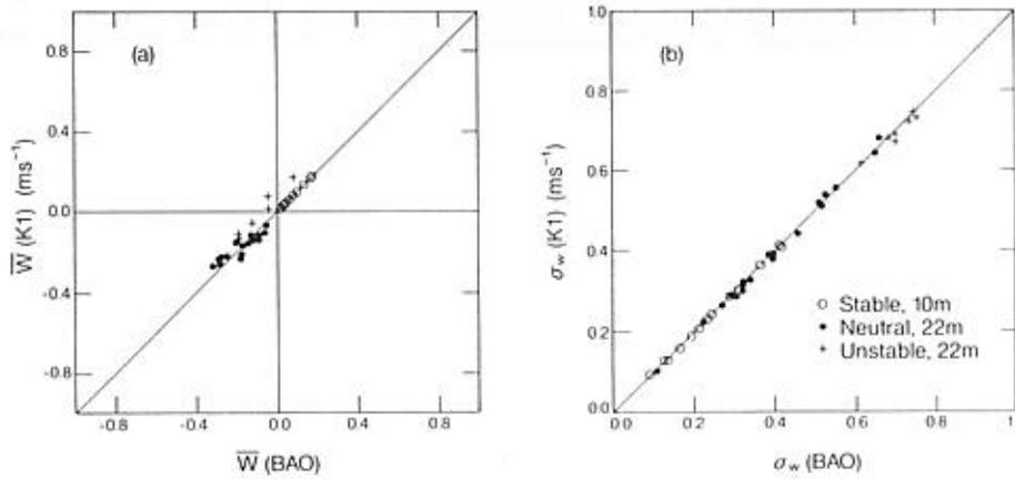
Fig. 4. Twenty-minute means and standard deviations of the vertical wind components measured by the BAO and KI probes.
