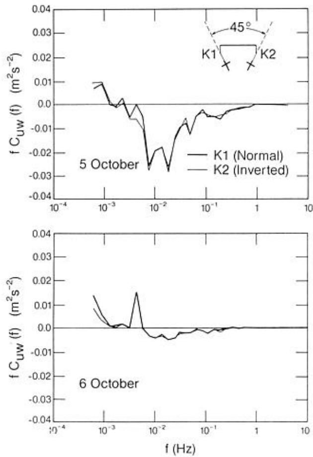
Fig. 9. One-hour cospectra from the slightly unstable (5 October) and slightly stable (6 October) periods in Test No. 2.
