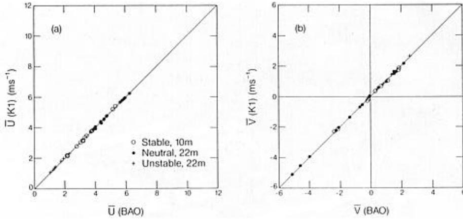
Fig. 3. Twenty-minute averaged horizontal wind components measured by the BAO and KI probes along their horizontal acoustic paths.
