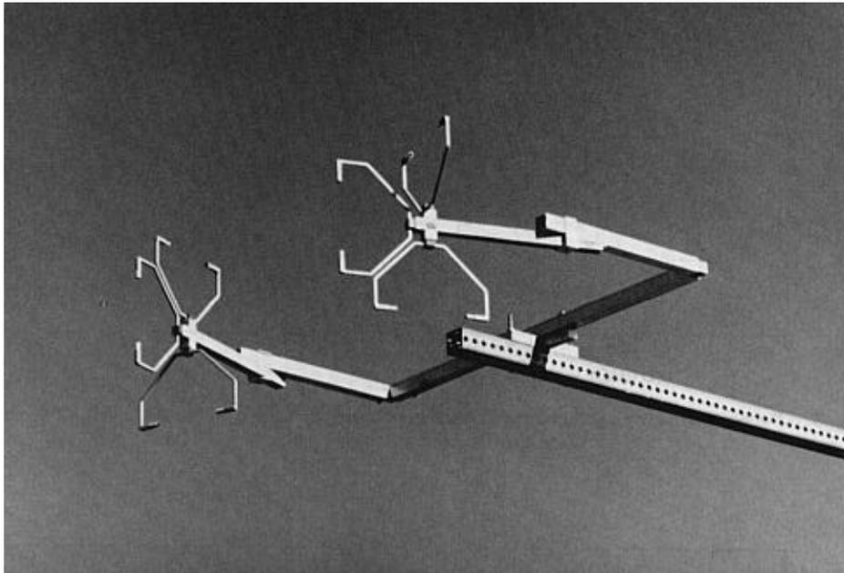
Fig. 2. New probes K1 (left) and K2 (right) turned  $22.5^\circ$  toward each other. K2 is inverted with respect to K1.
