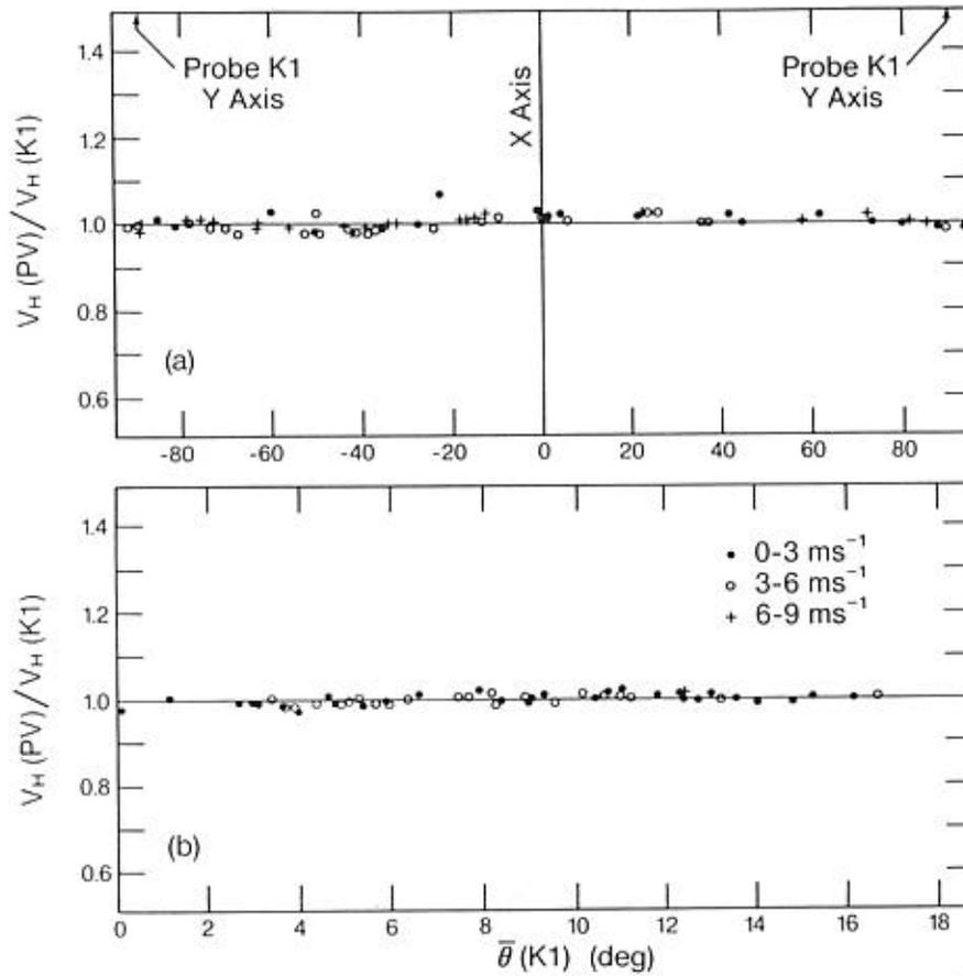
Fig. 6. Horizontal wind vectors measured by the propeller-vane anemometer and K1 probe:
