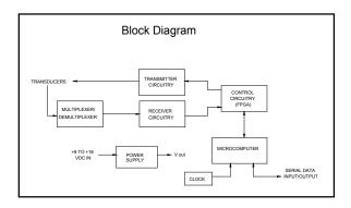
The basic system is DC powered (+9 to +18 VDC). Other power requirements can be accommodated, such as: 110 VAC/60Hz for North American applications, or 220 VAC/50Hz for International applications. (See Options List)
