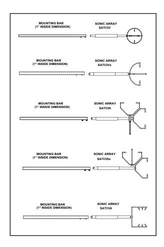
"A" Style Probe Assembly - nonorthogonal design ideal for higher wind speeds.
