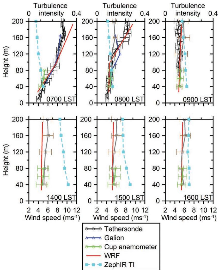
wind speed  $U_{\text{freestream}}$  is therefore in the range  $6.5\text{--}6.9 \text{ m s}^{-1}$ . Thus, the wake magnitude at this downwind distance (expressed as  $U_{\text{wake}}/U_{\text{freestream}}$ ) was 0.78–0.83 (where the range shows the variation in free-stream values). Employing the Wind Atlas Analysis and Application Program (WAsP) Park wake model (Barthelmie et al. 2009), a wake-decay coefficient of 0.075 and a thrust coefficient of 0.8 indicate the wake wind speed is
