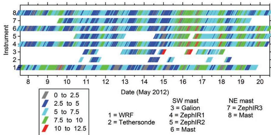
**FIG. 3.** Availability and magnitude of 10-min-mean wind speeds from the different instruments and WRF simulations during the experimental period. The colored bar indicates the wind speed at 80-m height ( $\text{m s}^{-1}$ ). The different rows show the instruments from which measurements are presented, so, for example, the row denoted “4” indicates wind speeds from the ZephIR located at the SW MM.
