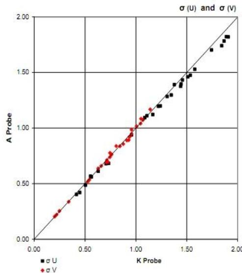
Figure 1. Scatter diagram of measured  $U$  and  $V$  standard deviations.
