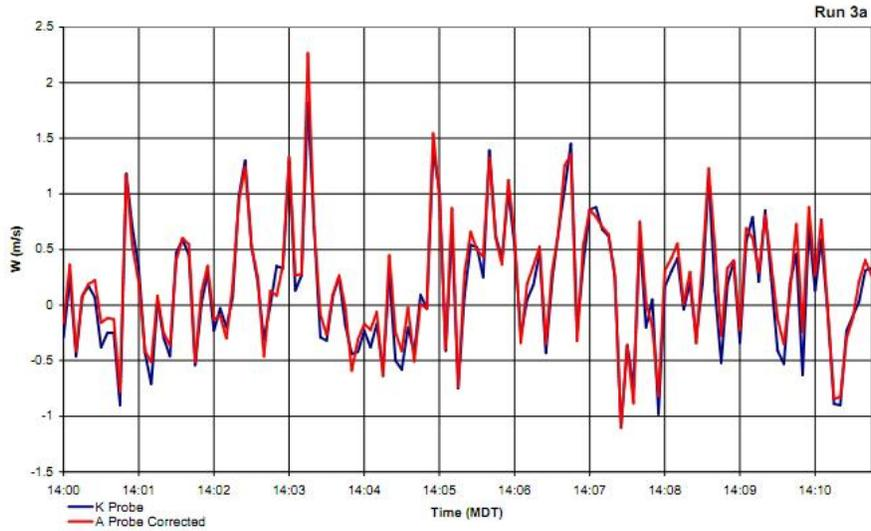
Figure 3(a). Plots of  $W$  with Eq. (1) correction on the A-Probe.
