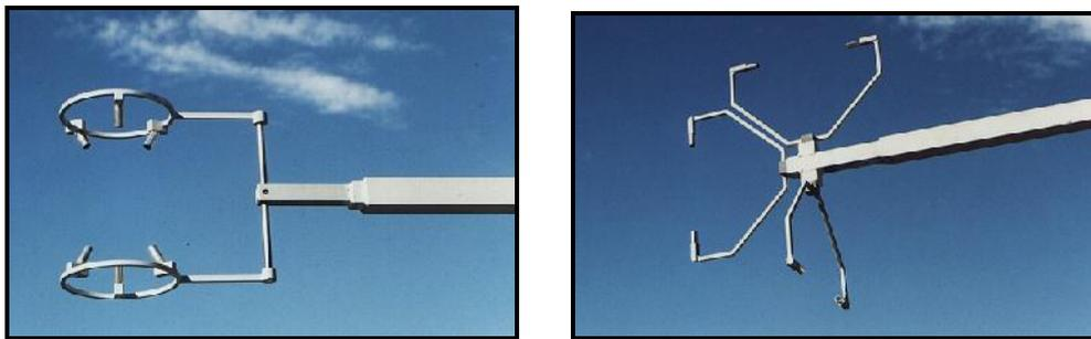
*Figures 2a and 2b - ATI's new non-orthogonal A-Probe and their K-Probe for inter-comparison tests*
