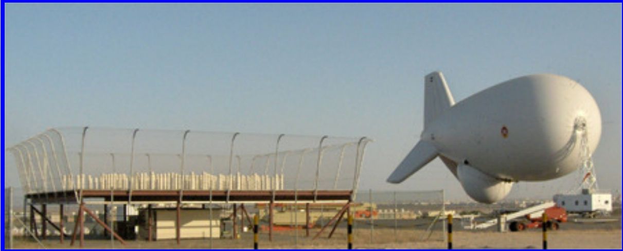
ATI's 192 element 449 MHz system installed in Kuwait for operational aerostat support.
